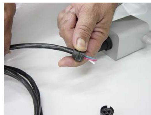
Figure 1.16 – Assembling the wire bracket
