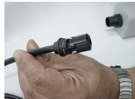
Figure 1.12 – Connector with the cable's wires maintained in their orifices
