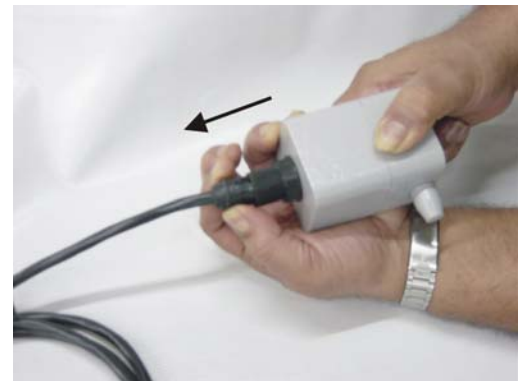
Figure 1.10 – Disconnecting the Hall sensor cable
