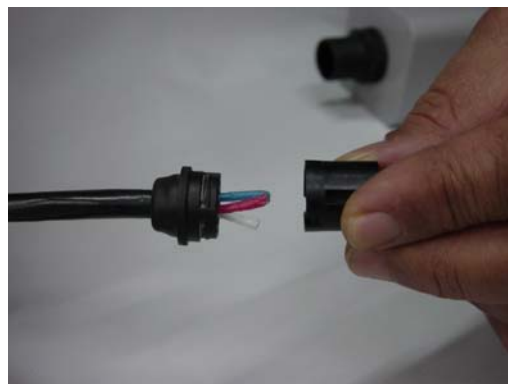
Figure 1.14 – Release the cables' connector
