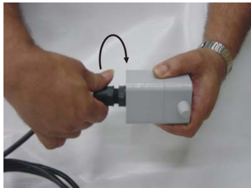
Figure 1.09 – Disconnecting the cover of the Hall sensor cable
