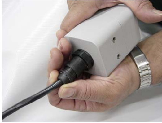
Figure 1.19 – Fasten the cover to the remote Hall
