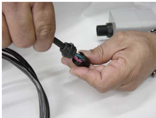
Figure 1.17 – Inserting the wires in the connector
